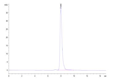
The purity of Biotinylated Human Nectin-4 IgV Domain is greater than 95% as determined by SEC-HPLC.
